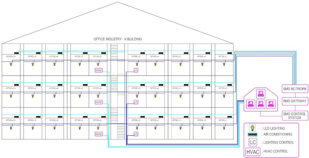
Figure 5. Topology BMS for lighting control.
